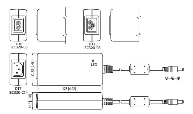
Notes: (1) The length of output cable should be 1040±50mm, 14AWG for 12V and 1980±150mm, 16AWG for 24-48V.
